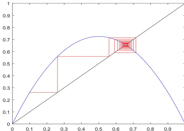
Figure 2.3: The cobweb diagram (or web plot) of the dynamical system defined by  $f(x) = 2.9x(1 - x)$ .
