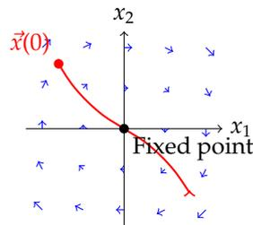
Figure 1.3: Phase portrait showing vector field (blue arrows) and a sample orbit (red curve) starting from  $\vec{x}(0)$
