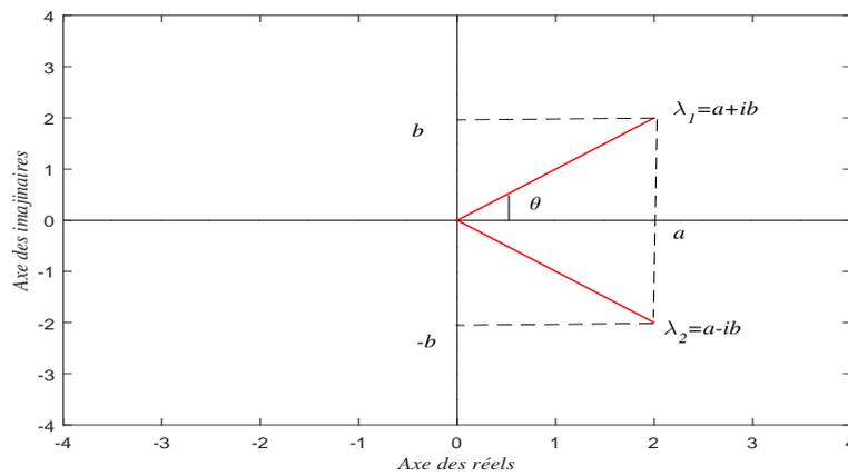
Figure 3.7: Geometric representation of the eigenvalues  $\lambda_{1,2} = a \pm ib = re^{\pm i\theta}$ .
