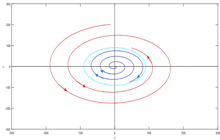
Figure 4.14: Supercritical Neimark–Sacker bifurcation. (a) Stable focus for  $\mu < \mu_0$ . (b) Stable closed invariant curve for  $\mu > \mu_0$ .
