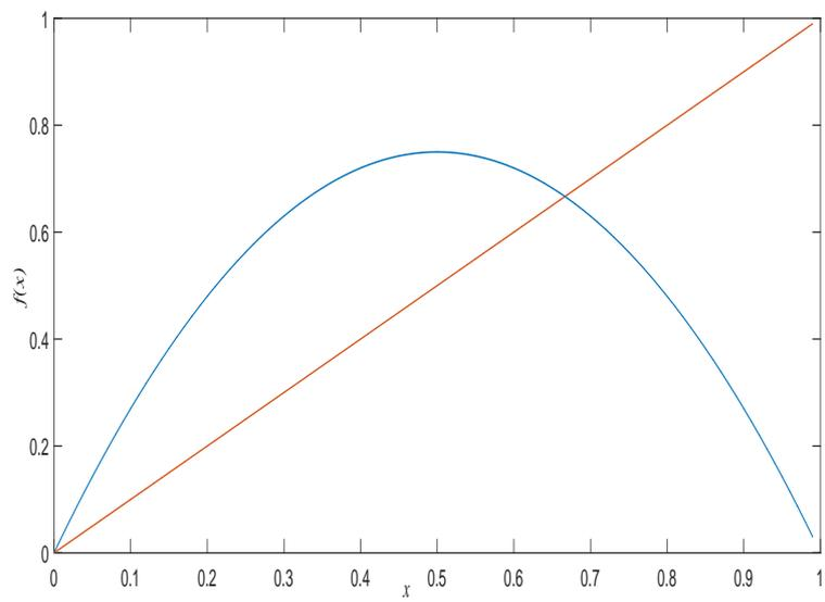
Figure 2.2: The fixed points of the mapping  $f(x) = 3x(1 - x)$ .
