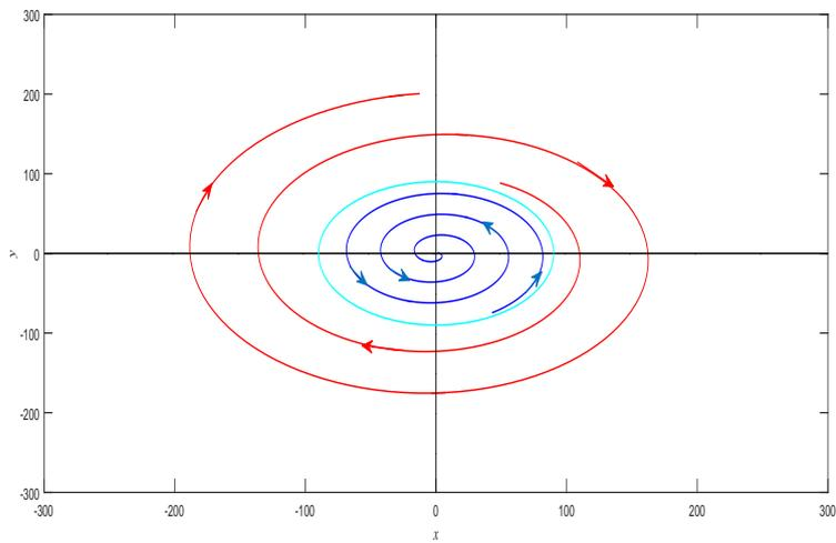
Figure 4.15: Subcritical Neimark–Sacker bifurcation. (a) Stable focus for  $\mu < \mu_0$ . (b) Unstable closed invariant curve for  $\mu > \mu_0$ .
