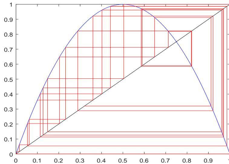
Figure 2.6: The cobweb diagram (or web plot) of the dynamical system defined by  $f(x) = 4x(1 - x)$ .
