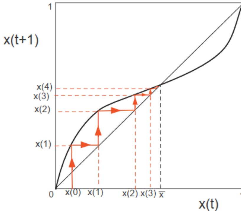
Figure 2.7: Graphical method to obtain a trajectory
