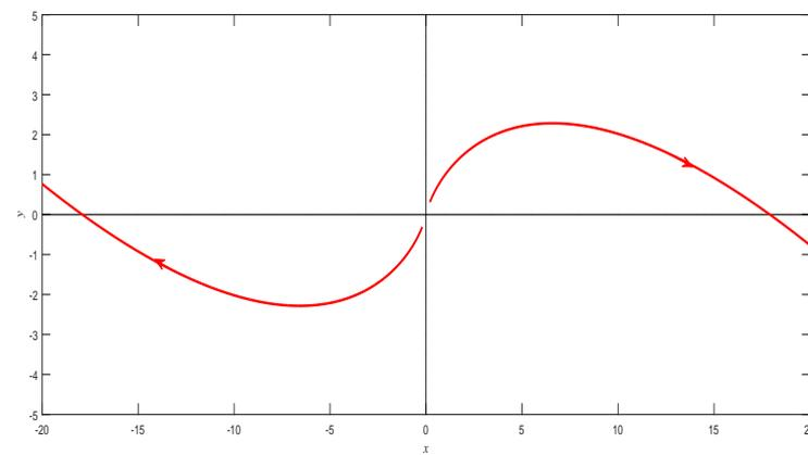
Figure 3.6: Phase portrait of the (3.12) if  $\lambda_1 = \lambda_2 = \lambda$  (a) Improper stable node  $0 < \lambda < 1$ . (b) Improper unstable node  $1 < \lambda < \infty$ .
