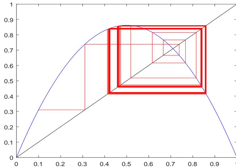
Figure 2.5: The cobweb diagram (or web plot) of the dynamical system defined by  $f(x) = 3.4495x(1 - x)$ .
