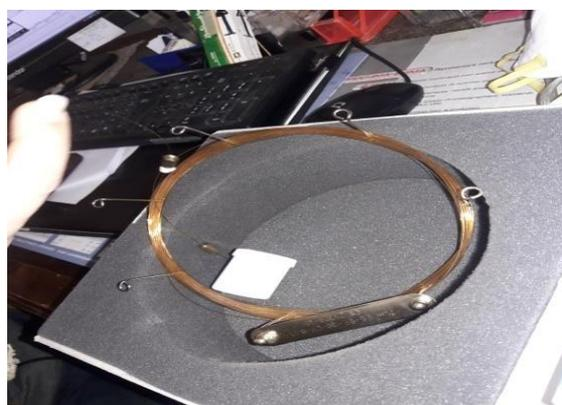
**Figure 13 :** Colonne capillaire S.N.V.Jijel.
