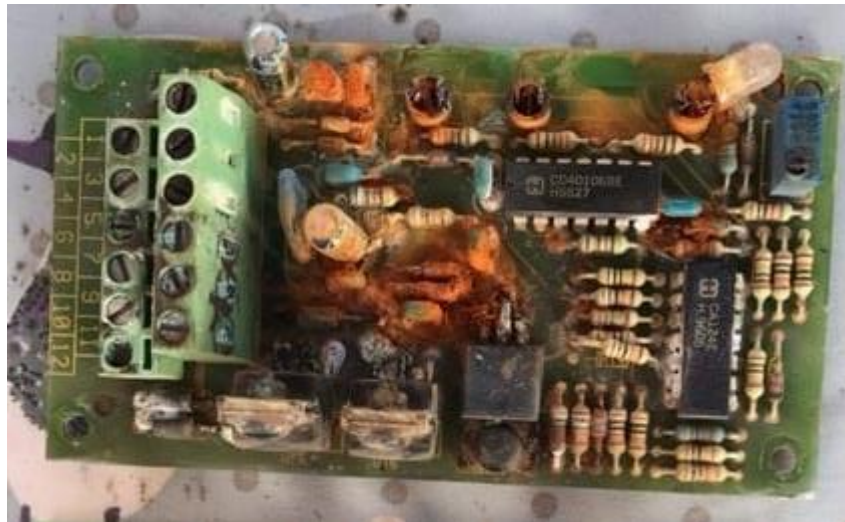
Figure II.38 : Risque de court-circuit. [33]
