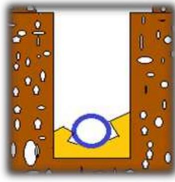
Figure 6 : Appui incorrect
