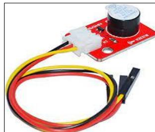
Figure 3. 5: Module Buzzer.
