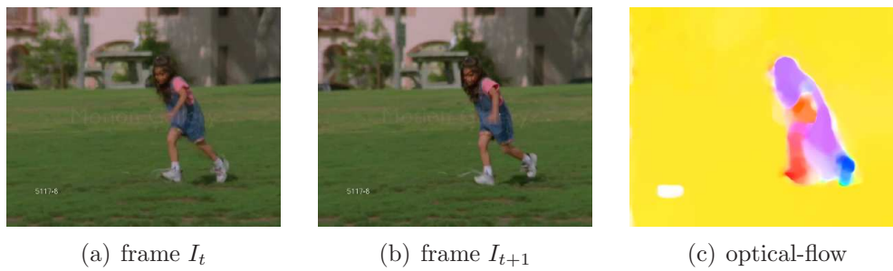
FIGURE 2.7: Illustration of the optical-flow feature. (a)-(b) input frames. (c) the resulting optical flow using the method in [4].
