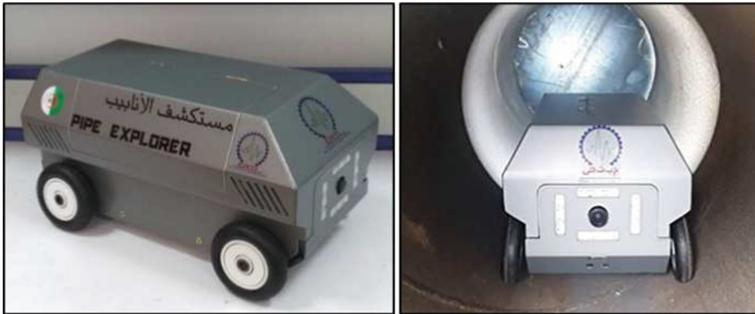
Fig. 2. The endoscope “Pipe-Explorer”
